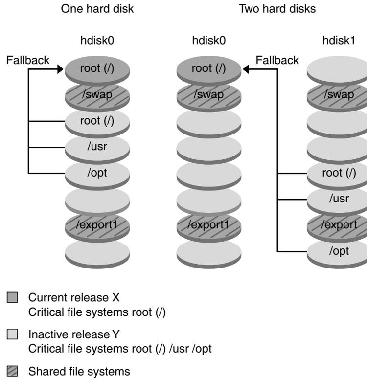
**FIGURE 30-7** Fallback to the Original Boot Environment
